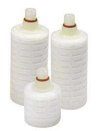
The use of a naturally hydrophobic membrane in **SupaPore TP** cartridges helps prevent the filter from wetting-out during use. This is critical in applications where water vapour is present to ensure that air flow into and out of the equipment is maintained. Typical applications include tanks containing liquids at elevated temperatures and autoclaves where steam may come into contact with the filter.
